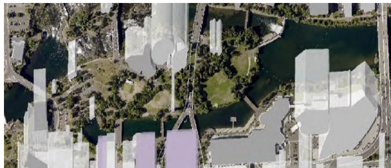
Existing shadows at noon on December 21 st in Riverfront Park from current buildings (in gray) and from buildings built according to current restrictions (in purple): the southern edge of Riverfront Park would already be shadowed in winter if built according to current policy.
