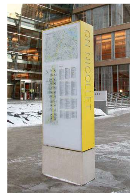
The wayfinding system for the Nicolett Ave corridor in Minneapolis, MN includes both full kiosks, and smaller elements that can be installed on poles for existing street lights, and traffic and pedestrian signals
