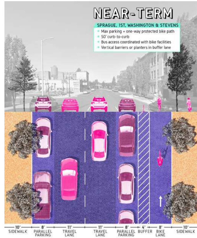
FIGURE 10 Cross-section of potential near term corridor improvements for Sprague Ave (West of Lincoln), 1st Avenue, and Washington and Stevens Streets. The location of protected bike lane will be impacted by the transit stops.
